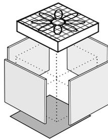
**ORIENT FILTERS & FAN SO THAT AIR FLOWS INTO SIDES & OUT TOP**
