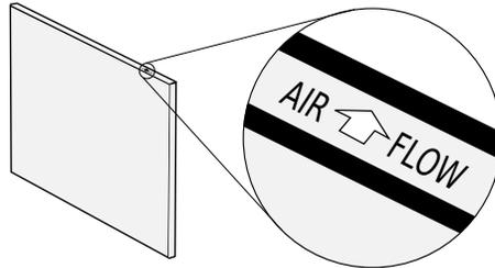
MERV 13 FILTERS HAVE A **PREFERRED AIRFLOW DIRECTION**, INDICATED ON FILTER FRAME
