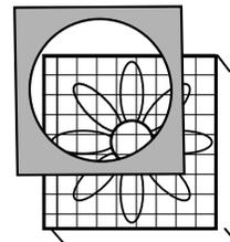
... WHICH CAN BE PREVENTED BY MAKING A **CIRCULAR SHROUD** FROM CARDBOARD SHEET (USING FAN DIAMETER)
