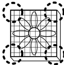
CORNERS OF BOX FAN CREATE 'BACK FLOW' CAN REDUCE PERFORMANCE...
